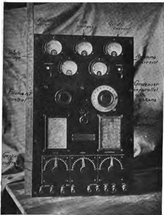
FIG. 63.—Front view of a small continuous-wave transmitter; the high-frequency power is generated by four five-watt tubes.
